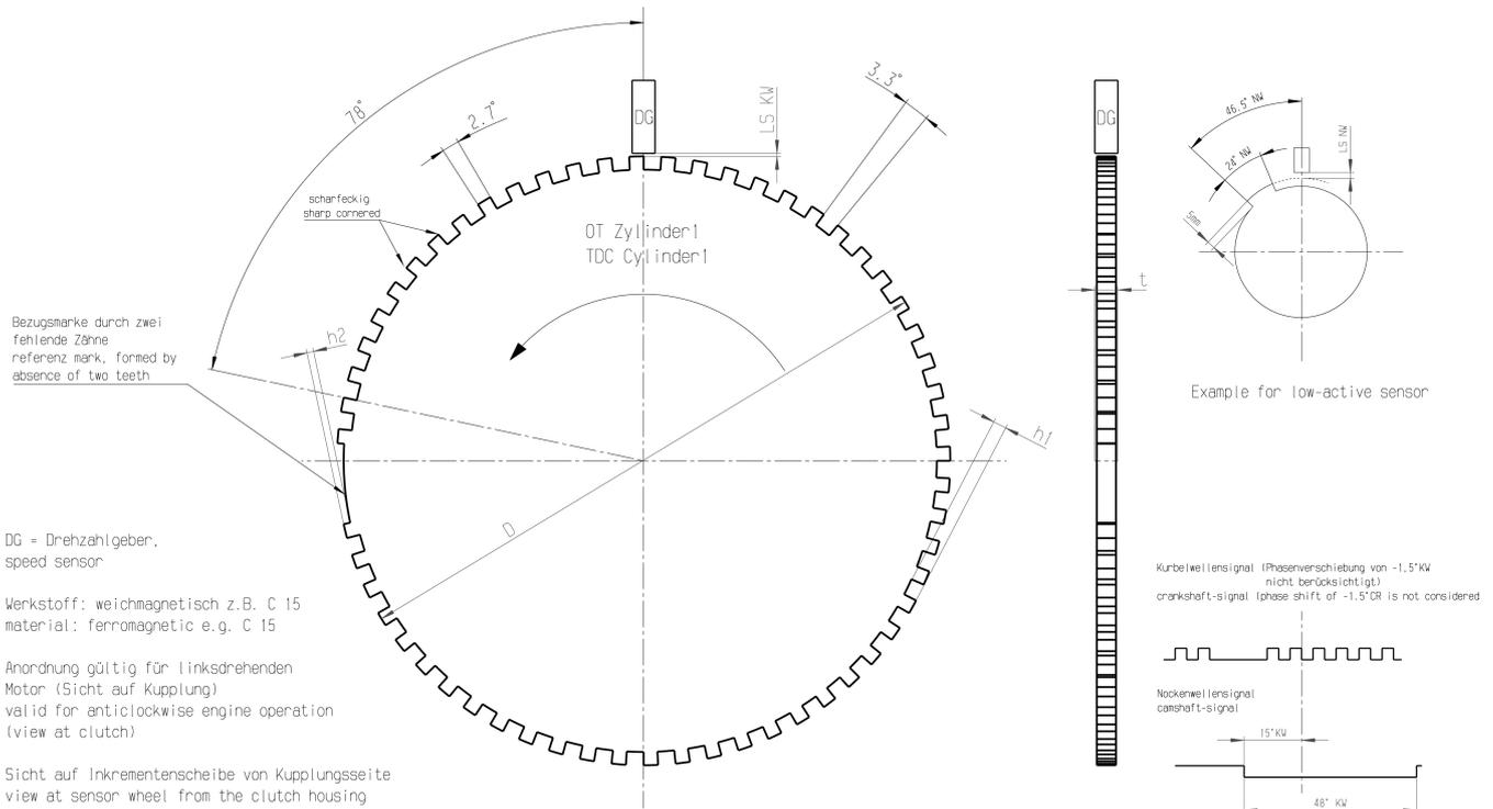
The procedure for correct adjustment of the trigger wheel
