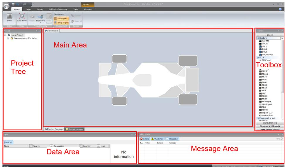
To create a new vehicle configuration, the devices can be pushed via drag & drop from the toolbox to the vehicle. Then they are part of the project and can be configured.
