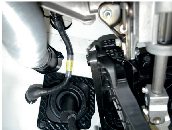
Illustration 23: ABS loom runs from connection point upwards
