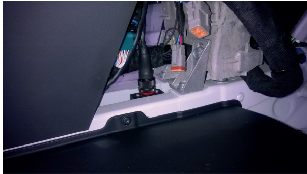
Illustration 19: Wheelspeed signal splitter with wiring loom plugged in
