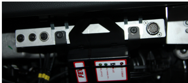
Illustration 20: Bracket with fuses and hole for ABS diagnostic plug in Gen. 2
