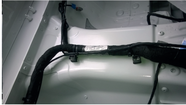
Illustration 25: ABS loom on top of center tunnel
