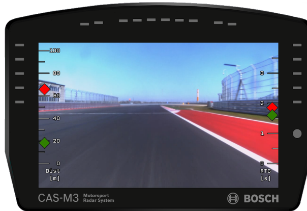
Illustration 6: Side gauges example
