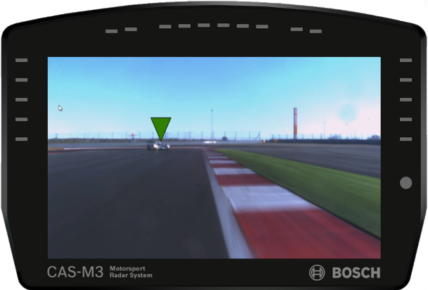
Illustration 4: Triangle vehicle marking
