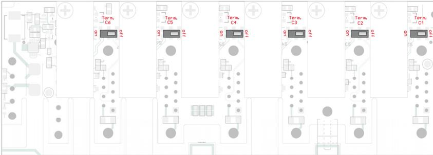
Figure 7: Positions of the switch blocks for CAN termination on the front board
