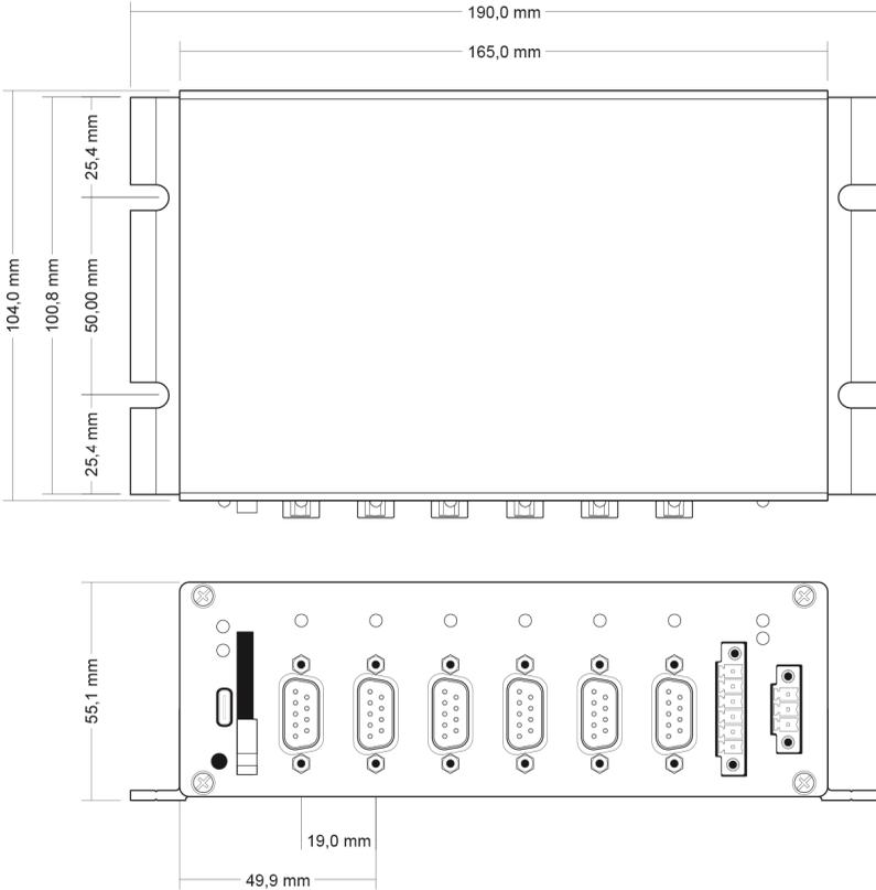
Figure 17: Dimension drawing PCAN-Router Pro FD
